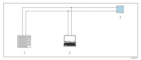
■ 57 Options for remote operation via Modbus-RS485 protocol (active)
