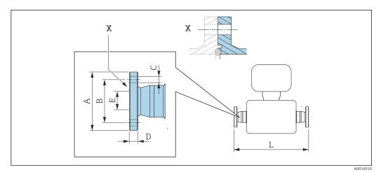
$\blacksquare$  31 Detail X: Asymmetrical process connection; the part shown in blue is provided by the supplier.
