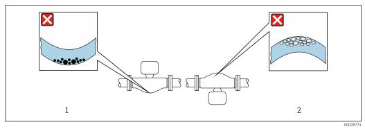
€ 18 Orientation of sensor with curved measuring tube
