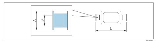
Length tolerance for dimension L in mm: +1.5 / -2.0
