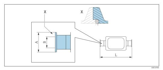
Detail X: Asymmetrical process connection; the part shown in blue is provided by the supplier.
