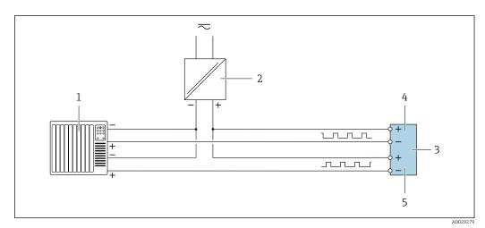
■ 13 Connection example for double pulse output (passive)
