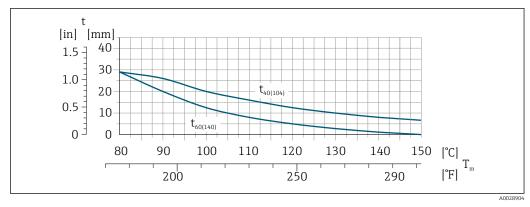
■ 29 Maximum recommended insulation thickness depending on the temperature of the medium and the ambient temperature
