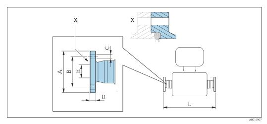
■ 43 Detail X: Asymmetrical process connection; the part shown in blue is provided by the supplier.
