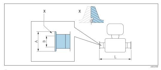
$\blacksquare$  35 Detail X: Asymmetrical process connection; the part shown in blue is provided by the supplier.
