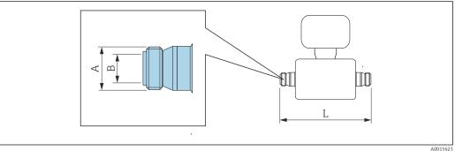
Length tolerance for dimension  $\boldsymbol{L}$  in mm: +1.5 / -2.0
