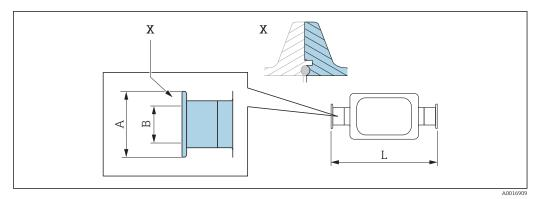
$\blacksquare$  38 Detail X: Asymmetrical process connection; the part shown in blue is provided by the supplier.
