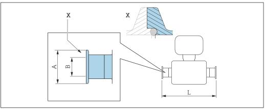
Detail X: Asymmetrical process connection; the part shown in blue is provided by the supplier.
