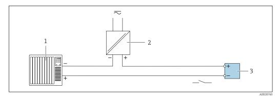
■ 11 Connection example for switch output (passive)
