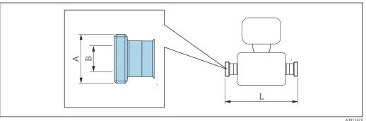
Length tolerance for dimension L in mm:  $+1.5 \ / \ -2.0$
