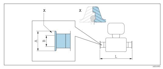
$\blacksquare$  34 Detail X: Asymmetrical process connection; the part shown in blue is provided by the supplier.
