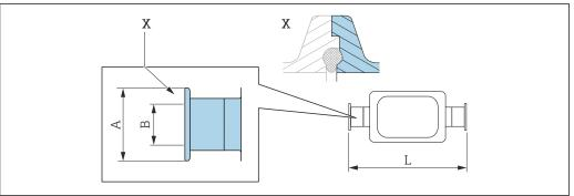
Detail X: Asymmetrical process connection; the part shown in blue is provided by the supplier.
