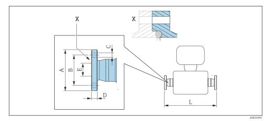
**■** 32 Detail X: Asymmetrical process connection; the part shown in blue is provided by the supplier.
