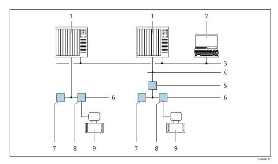
$\blacksquare$  55 Options for remote operation via FOUNDATION Fieldbus network
