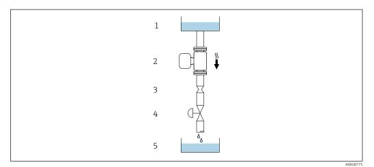
$\blacksquare$  17 Installation in a down pipe (e.g. for batching applications)
