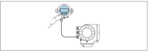
■ 52 Operation via remote display and operating module DKX001
