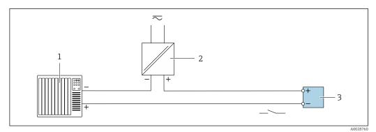
■ 14 Connection example for relay output (passive)
